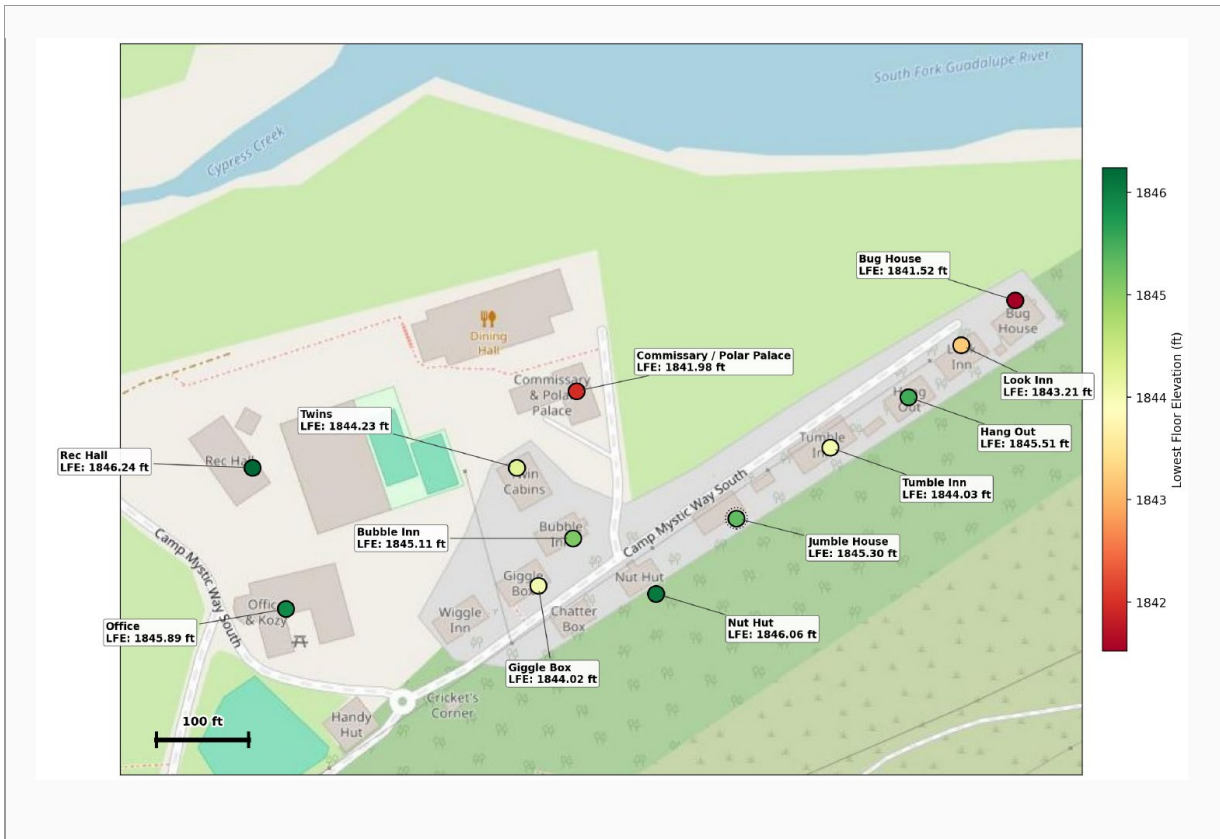
Figure A-2. Map of selected buildings at Camp Mystic Guadalupe River, with elevations.
